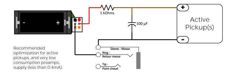
Option: filtered wiring for active pickups
